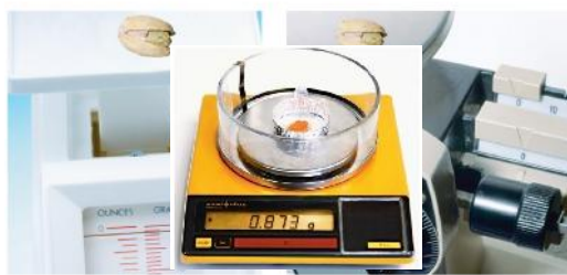
(a) Markings every 1 g Estimated reading 1.2 g
